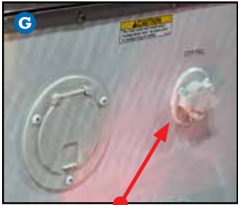
The city fill is located beneath the mechanical closet door side.
